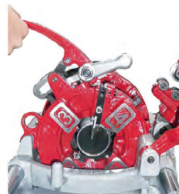
NV-auto Die-head (for 1/2"-2" pipe) NP80AV/AVIII
