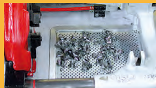
Fig. 2 Chips from roll threads
