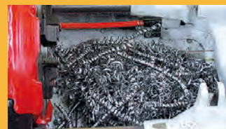
Fig. 1 Chips from cut threads
