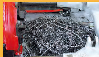
Fig. 1 Chips from cut threads
