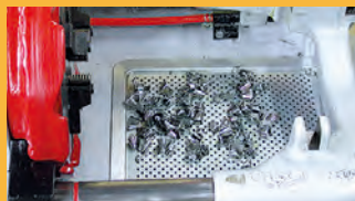
Fig. 2 Chips from roll threads
