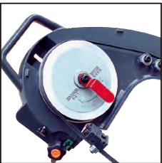
Fig. 2 Easy replacement of spare saw blade
