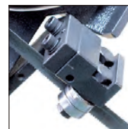
Fig. 11 Larger bearings provide greater durability.
