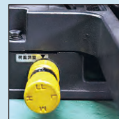
Fig. 8 Cutting Load Adjuster (LL, L, M, H)
