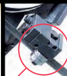
Fig. 3 Larger bearings provide greater durability
