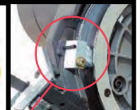
Fig. 5 Brush prevents blade slip from plastic wastage
