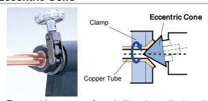
The eccentric cone moves forward with a rotary motion to gradually push and expand the inner diameter of the copper tube. The forward movement of the cone is then stopped by the clutch, which activates at a predetermined pressure. The flared surface of the copper tube is given a clean finish by the cone's rotary motion.
