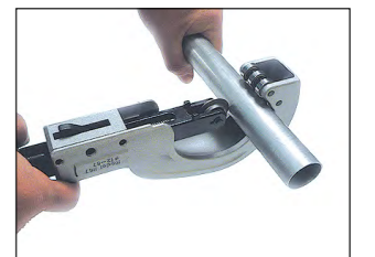
Cutting a short pipe Fig 4
